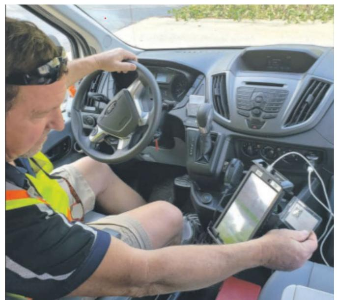
Transit operator John Roberts uses an onboard tablet to scan a payment card that automatically charges the fare amount and reduces the balance of the card
